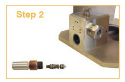
Align lobe on cartridge assembly with groove in cartridge holder and Turn counter clockwise to unlock and remove.
