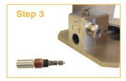
Replace cartridge and install in block
